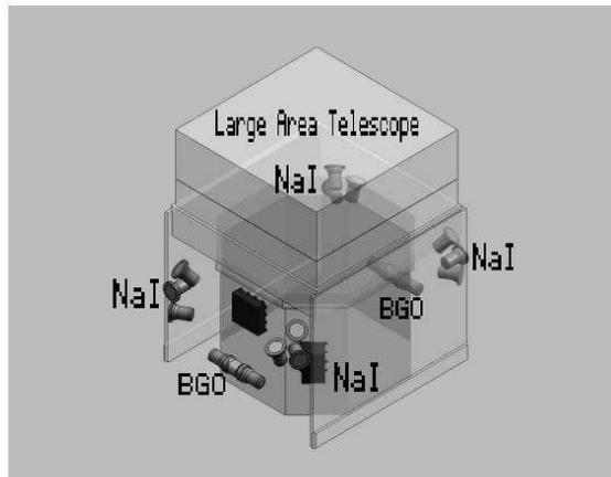
**FIGURE 1.** Placement of 12 NaI( $T\ell$ ) and 2 BGO detectors onboard the satellite with respect to LAT, shown as the large structure above the spacecraft structure.
